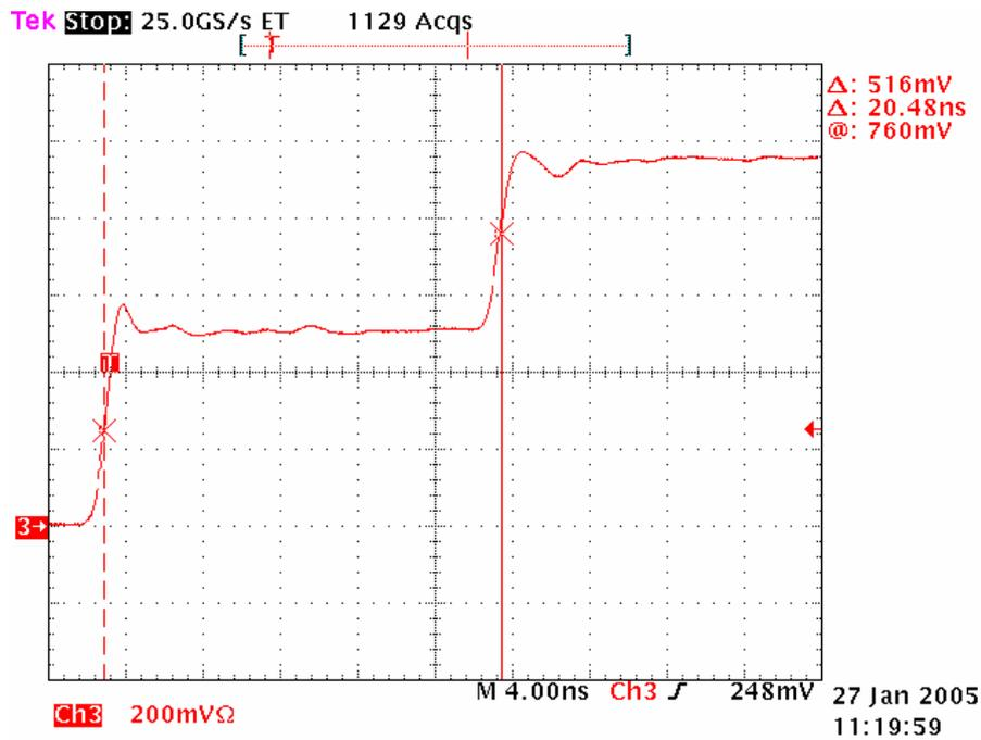
Figure 15: Adapted source resistance: picture created by the scope.
