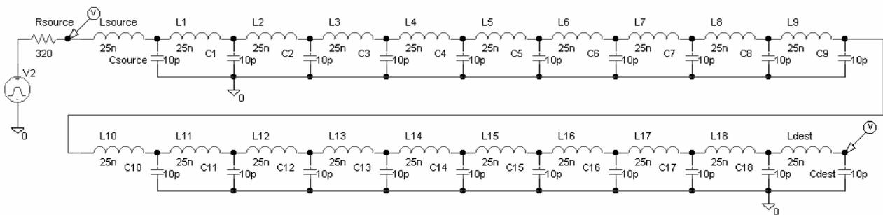
**Figure 8: Transmission line simulates by PSpice.**
