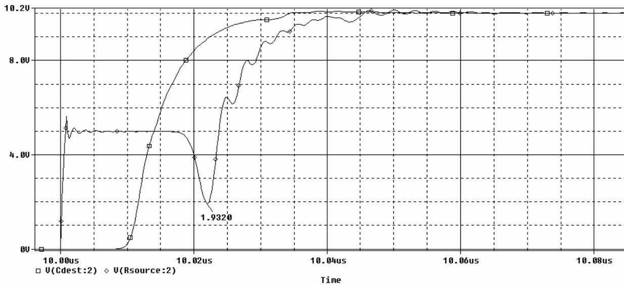
Figure 19: Capacitively terminated transmission line simulates by Pspice.
