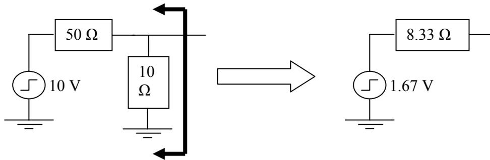
Figure 11: Thevenin equivalent circuit for the small input resistance.
