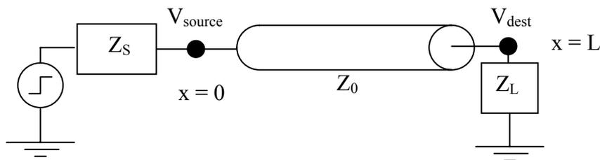
**Figure 2: Transmission line with terminating impedance.**
