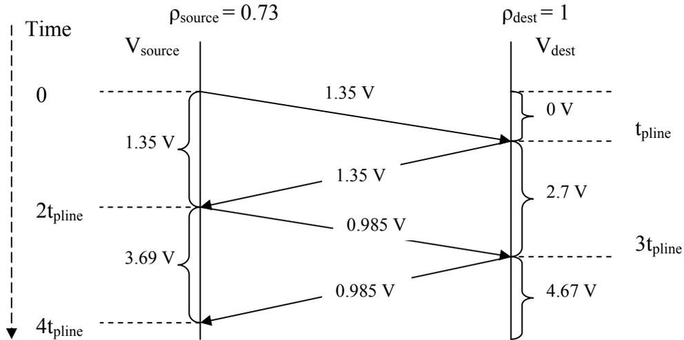
Figure 5: Lattice diagram for the large source resistance test.
