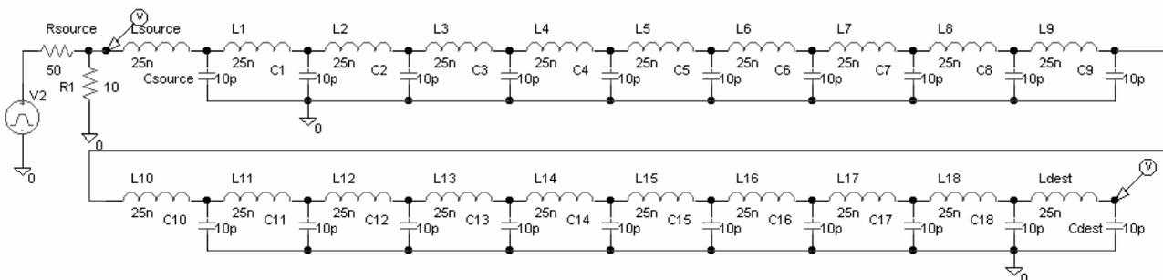
Figure 10: Transmission line with small source resistance simulates by PSpice.
