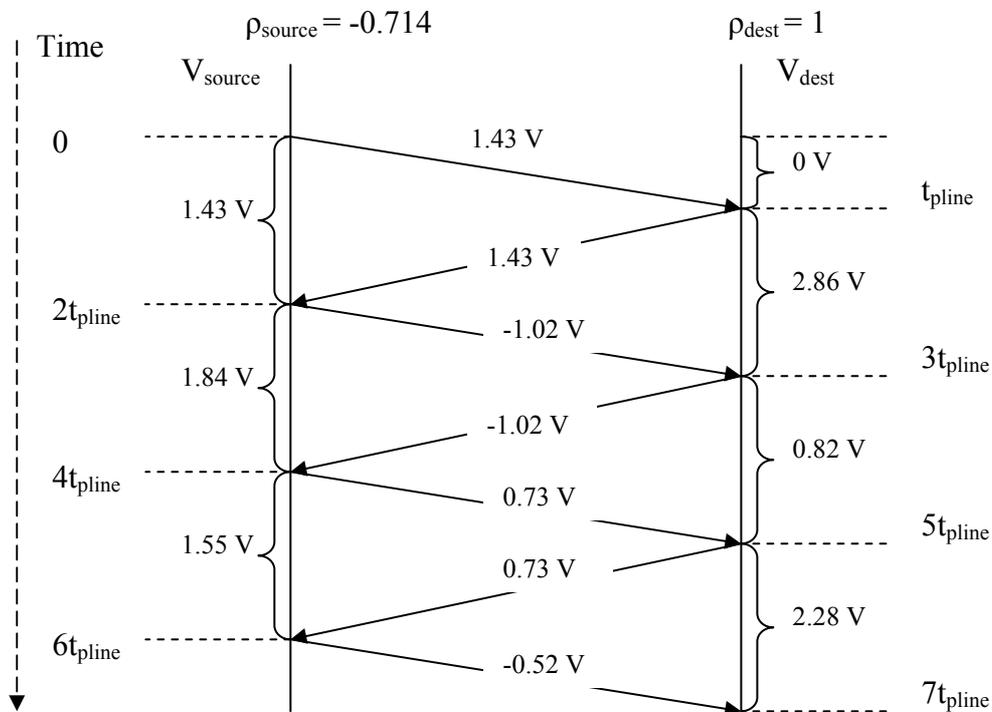
Figure 12: Lattice diagram for the small source resistance test.
