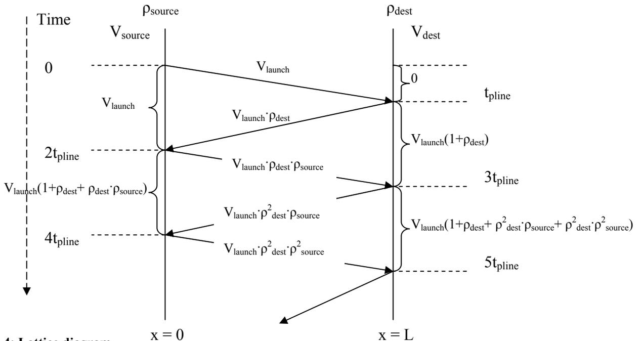
Figure 4: Lattice diagram
