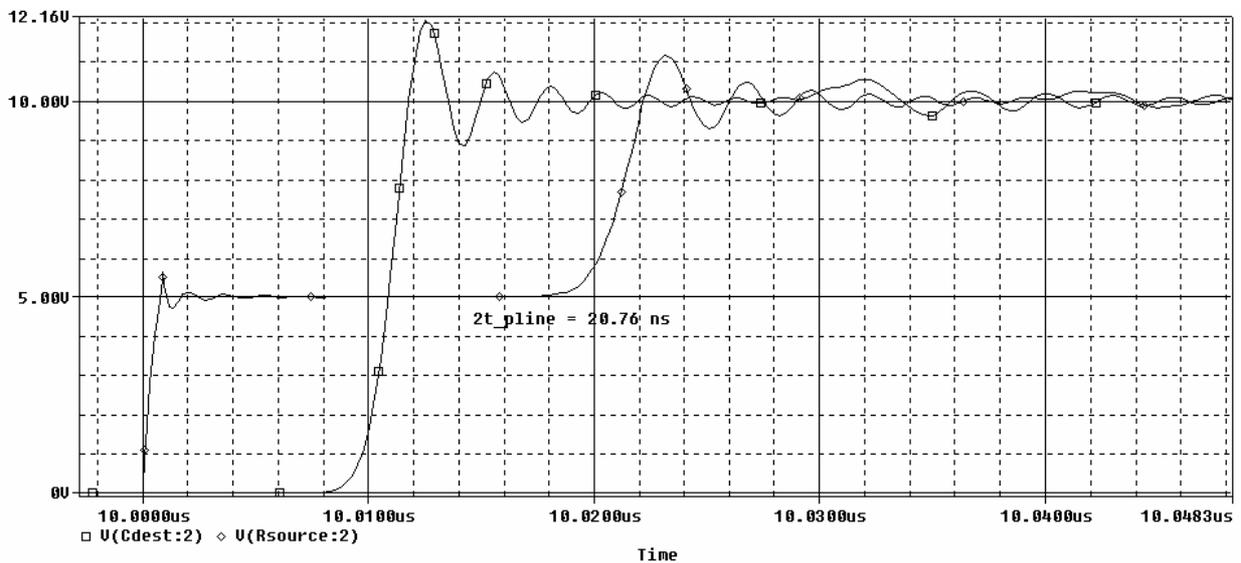
Figure 16: Source and destination voltage for adapted source resistance test made by PSPICE simulator.
