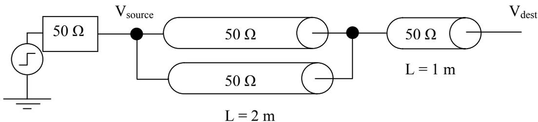
Figure 20: Series of two transmission line: circuit under test.
