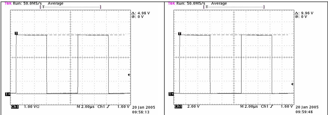
Figure 3: right – scope input impedance adapted to 50 Ω; left – scope input impedance equal to 1 MΩ.
