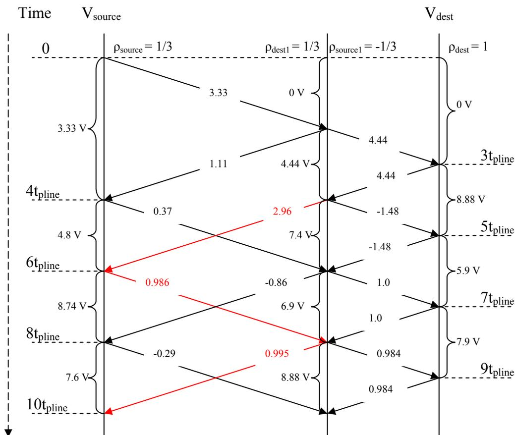
Figure 21: Series of two transmission line with different characteristic impedance: lattice diagram.
