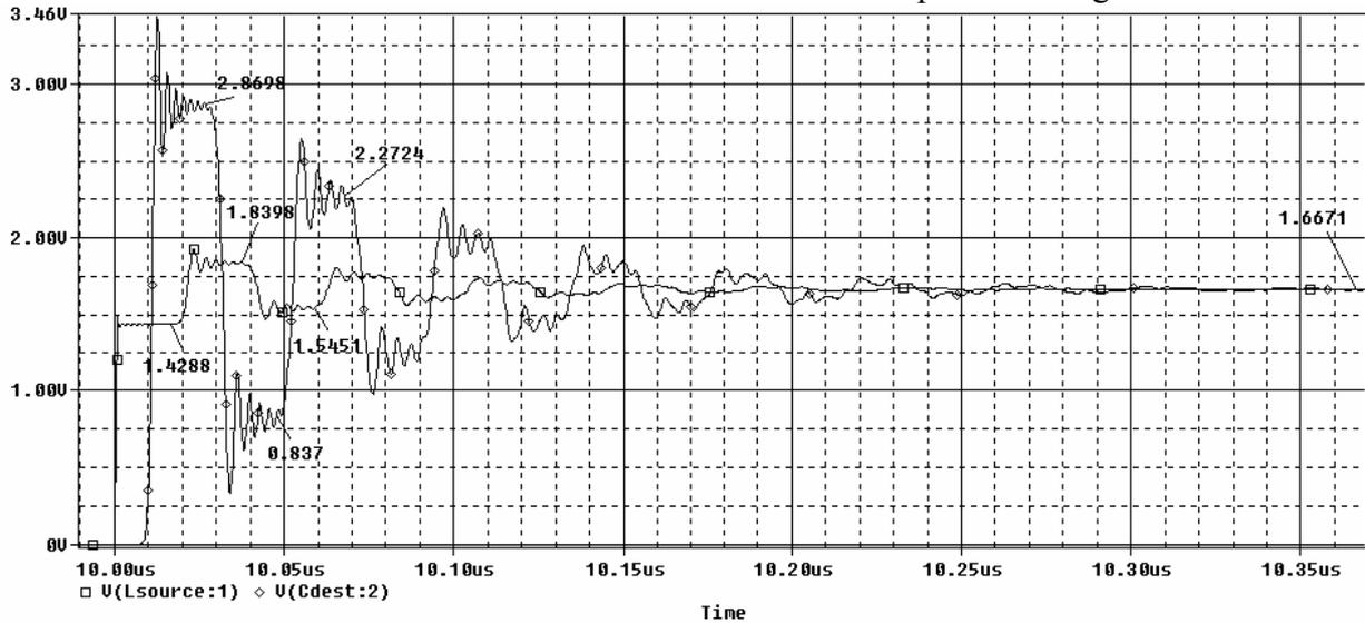
Figure 14: Source and destination voltage for small source resistance test make by PSpice simulator.
