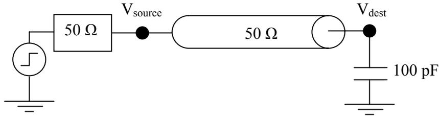
Figure 17: Transmission line terminates with a capacitive load.
