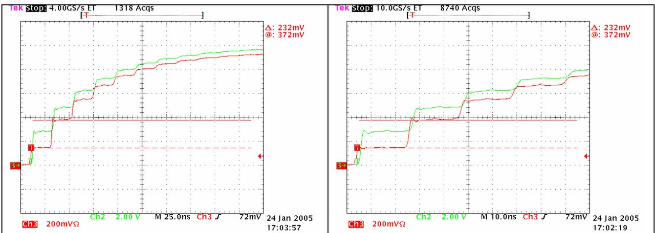
Figure 6: Large source resistance: picture create by the scope. Left picture is a zoom of the right one.
