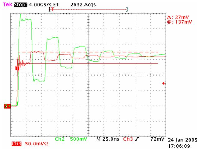
Figure 13: Small source resistance: picture creates by the scope.
