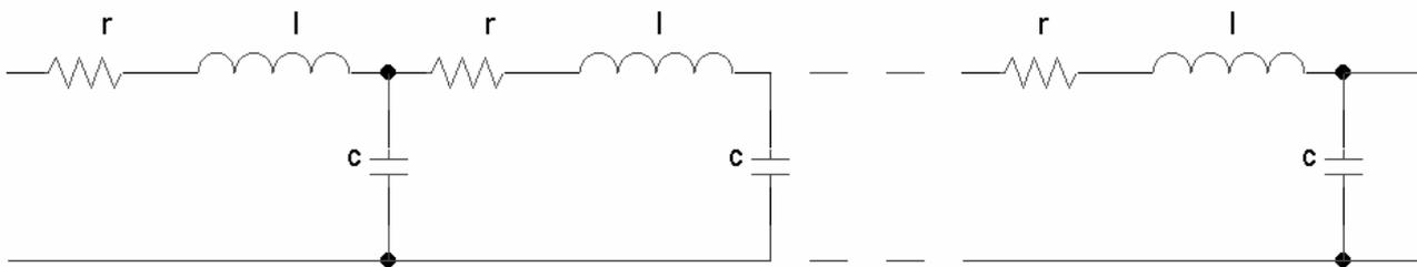
**Figure 1: Transmission line model**
