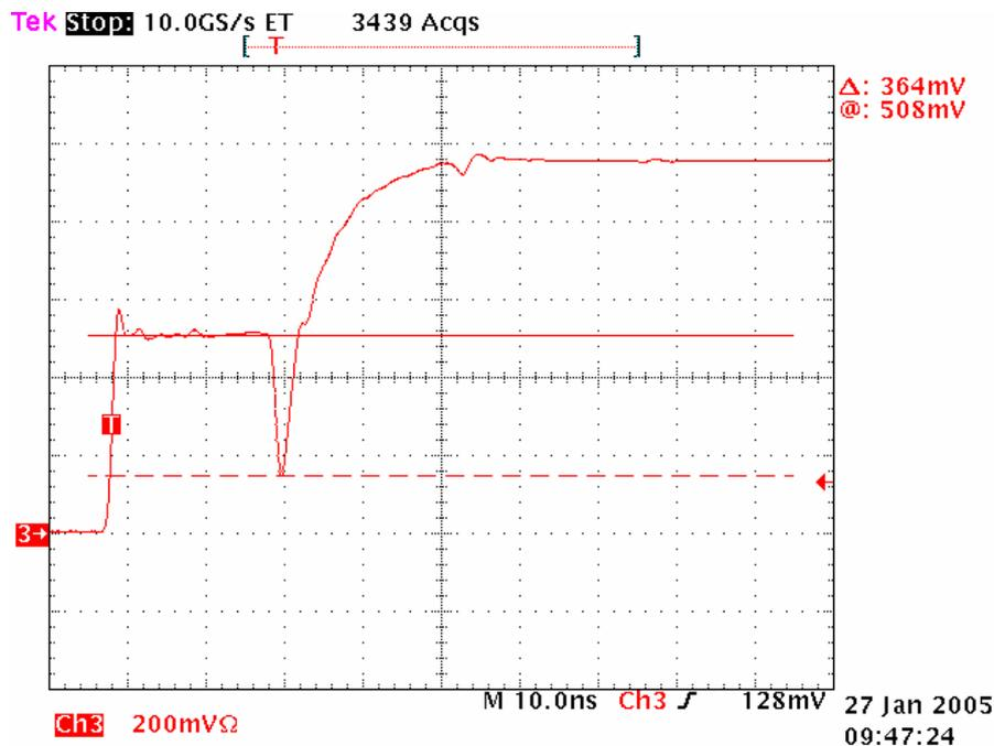
Figure 18: Capacitively terminated transmission line.
